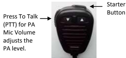
2. If the system does not respond to pressing the starter button and continues to cycle through the different tones, check the trigger switch is up (Int) and the microphone is properly plugged in
